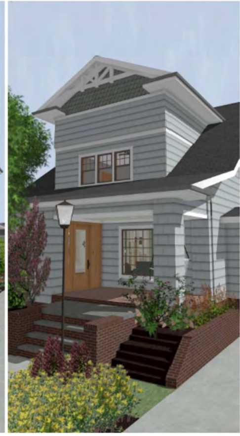
no bump out Even with flair/drip-edge above the second floor decorative trim board, it looks too flat and what is essentially a single layer makes it look taller and narrower.
