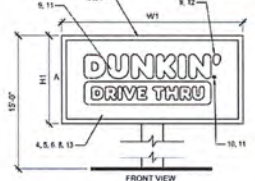
3 NEW SIGN- PYLON TYPE 1/4" = 1'-0" NOTE
