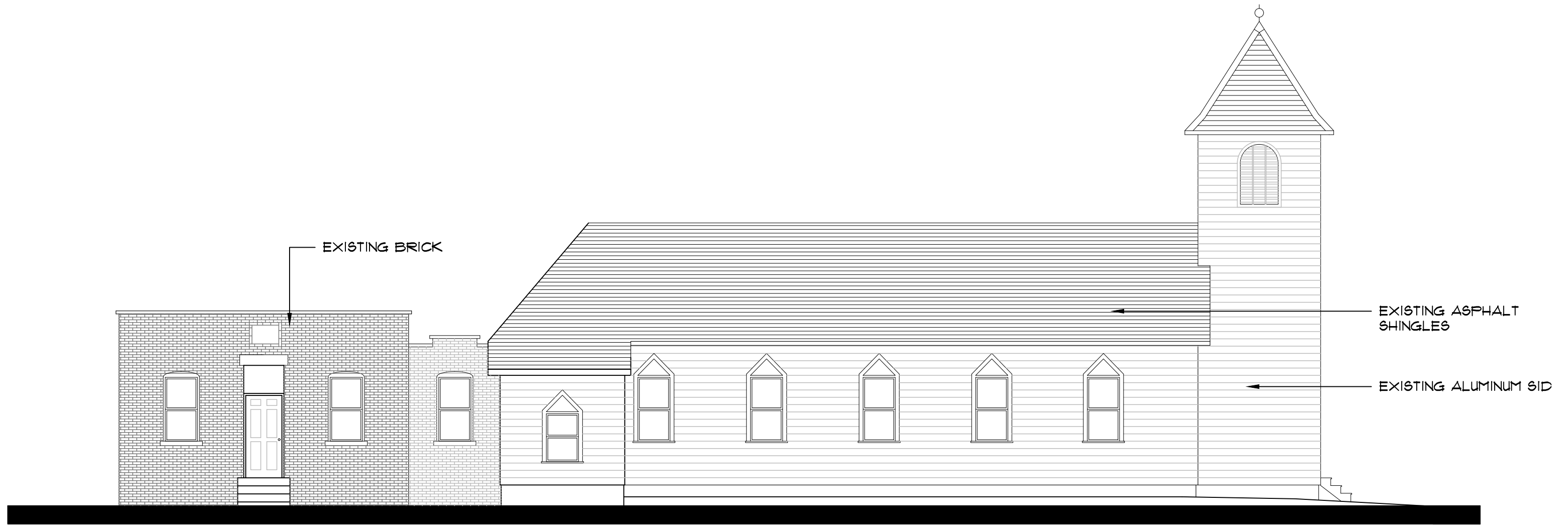
Existing Side Elevation 1/8" = 1'-0"
