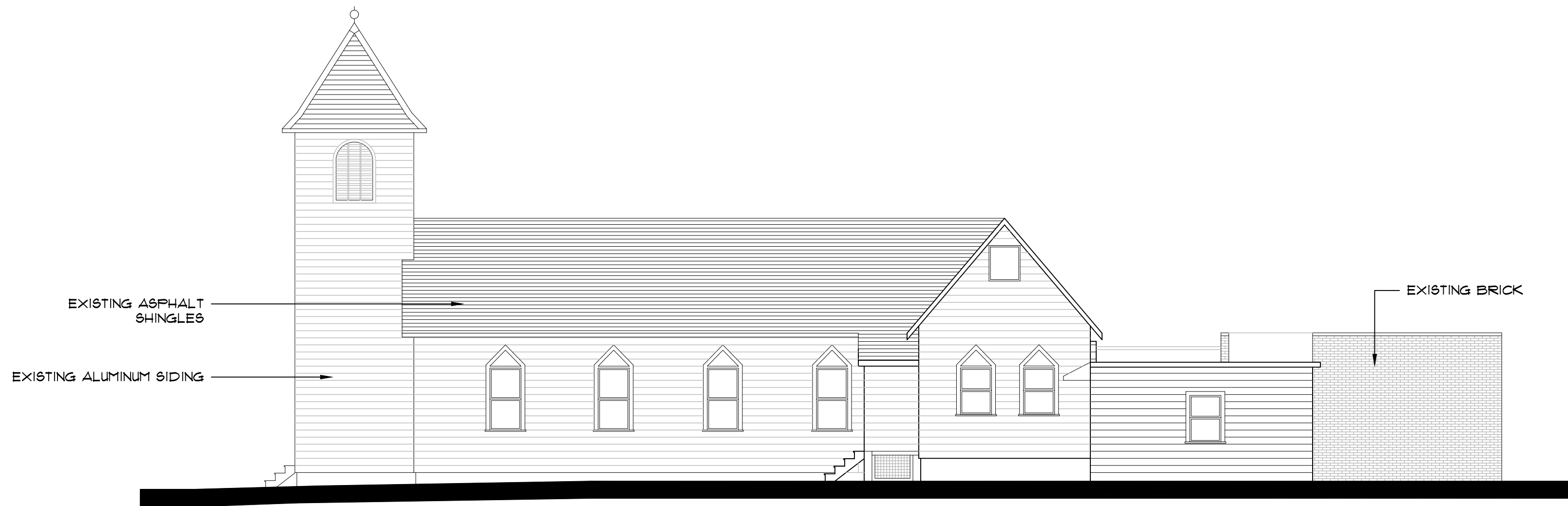
Existing Side Elevation 1/8" = 1'-0"
