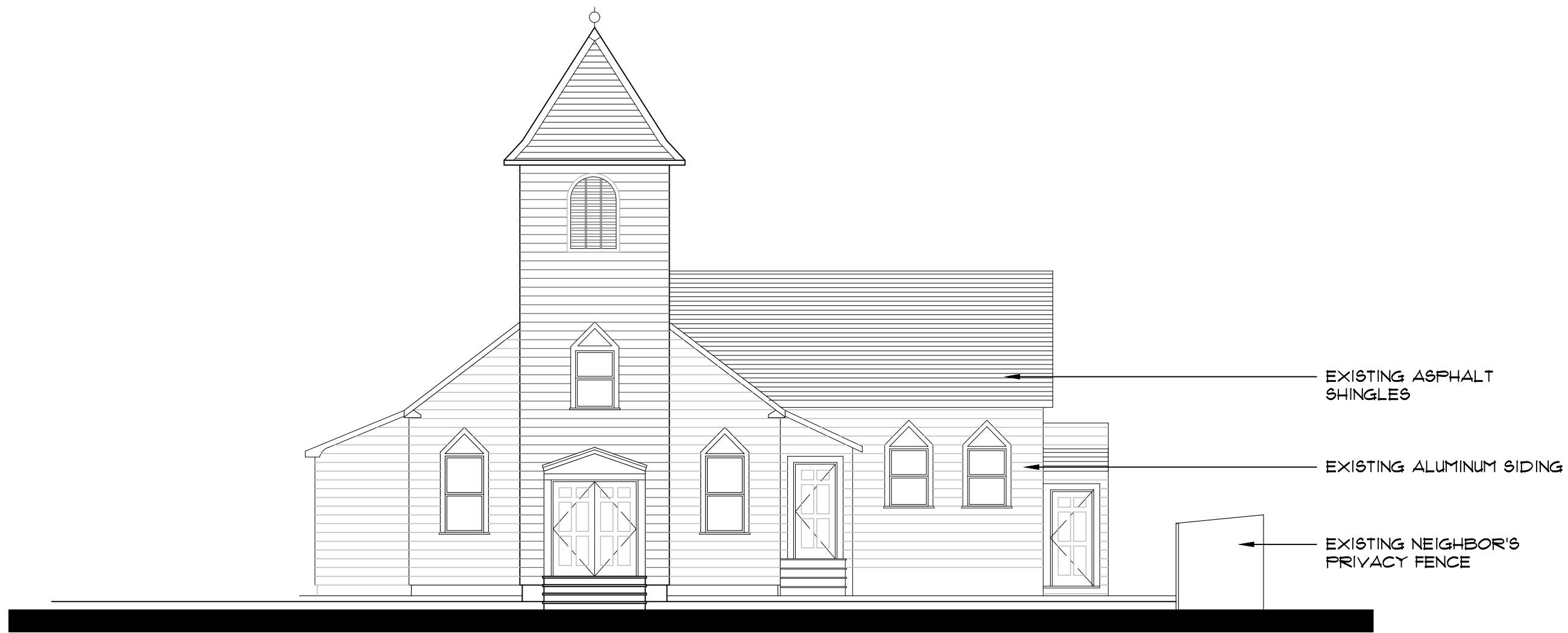
Existing Front Elevation 1/8" = 1'-0"
