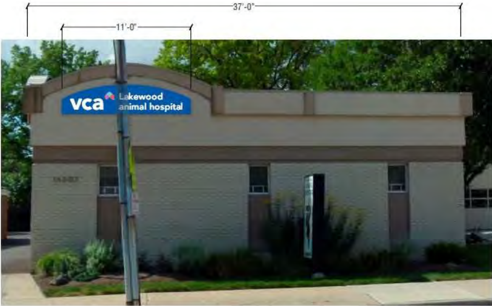
2 PROPOSED NEW NON-ILLUMINATED REVERSE PAN SIGN SCALE: 3/16" = 1'-0"
