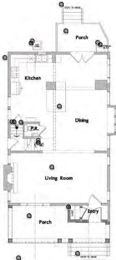
First Floor Plan SCALE 1/8" = 1'-0" ● SQ. FT. - EXISTING FIRST FLOOR ● SQ. FT. - EGRESS ADDITION ● SQ. FT. - FIRST FLOOR (TOTAL) ● SQ. FT. - FRONT PORCH ADDITION (NOT INCLUDED) ● SQ. FT. - TOTAL
