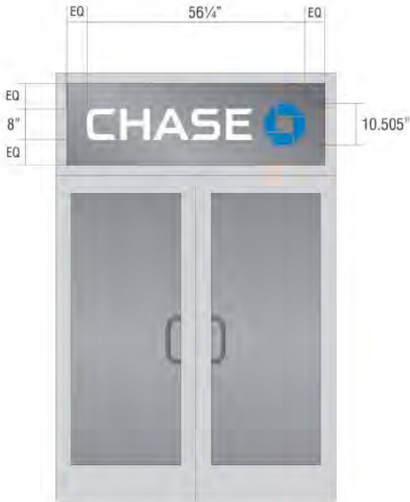
TYPICAL ENTRY DOOR SCALE: 1/2" = 1'-0"
