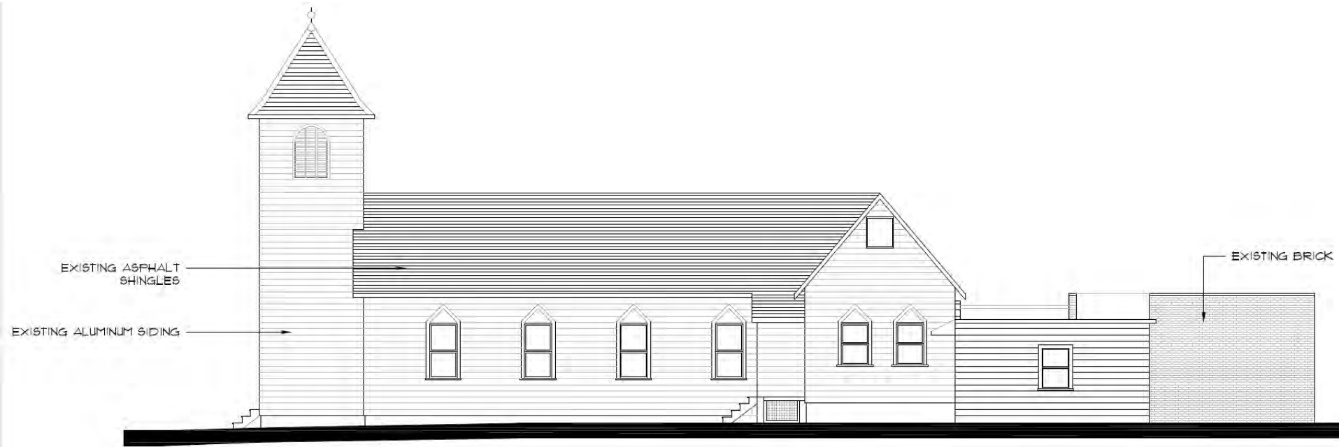
Existing Side Elevation 1/8" = 1'-0"
