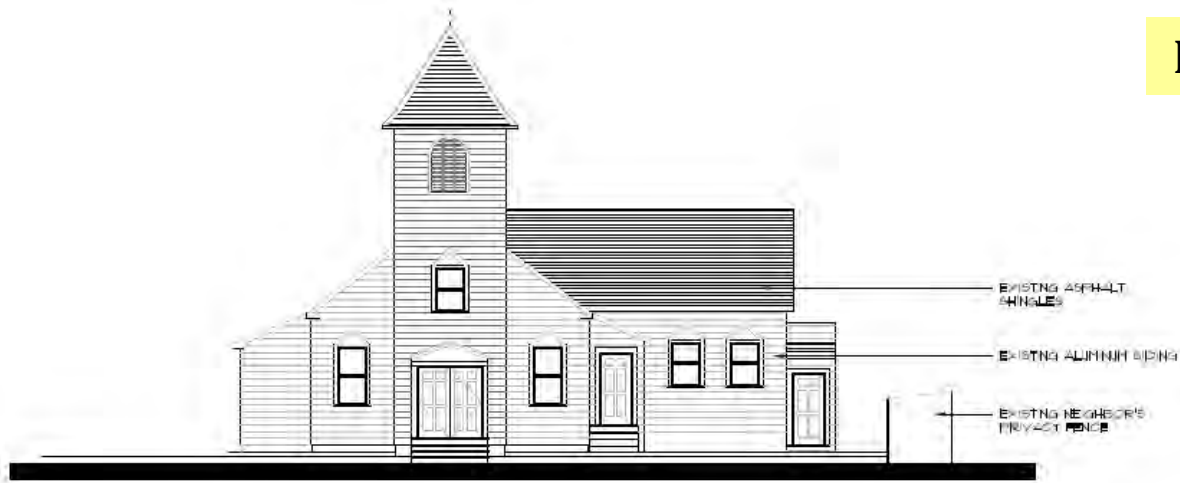
Existing Front Elevation 1/8" = 1'-0"
