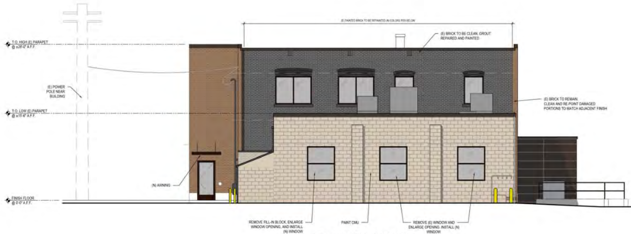
2 NORTH ELEVATION SCALE: 3/16" = 1'-0"
