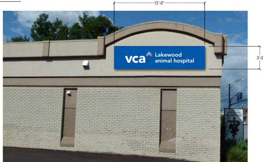
2 PROPOSED NEW NON-ILLUMINATED REVERSE PAN SIGN SCALE: 1/4" = 1'-0"
