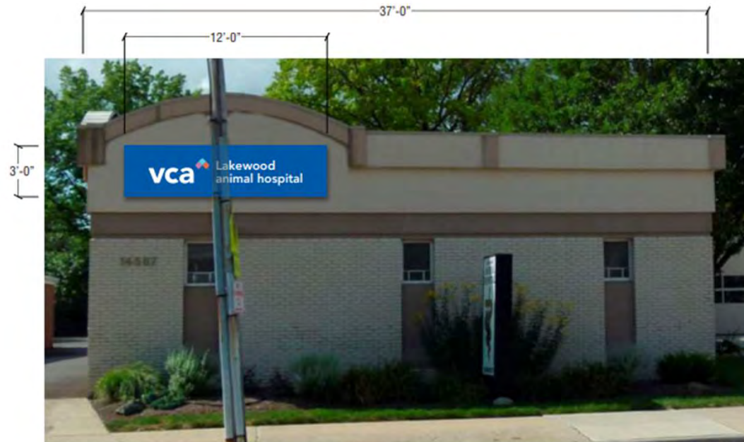
2 PROPOSED NEW NON-ILLUMINATED REVERSE PAN SIGN SCALE: 3/16" = 1'-0"
