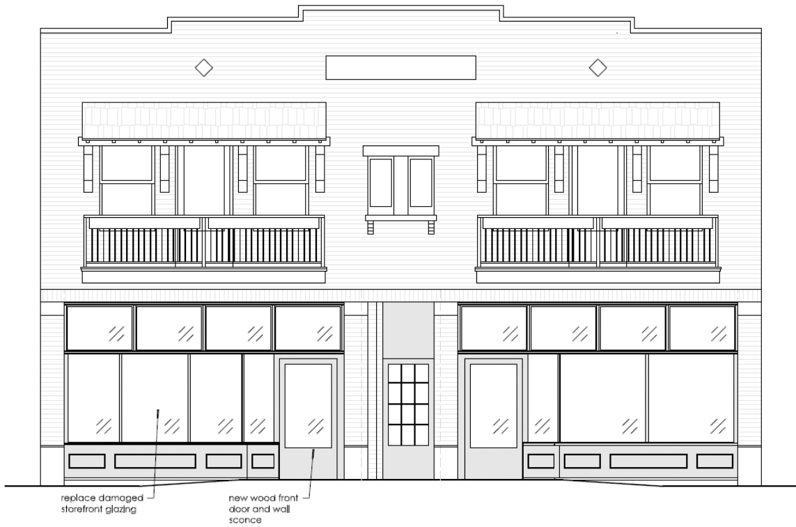
1 NEW ELEVATION ABR02 1/4" = 1'-0"
