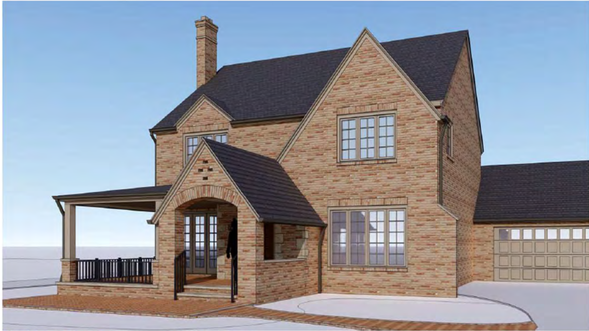
HIP ROOF - Asphalt Shingle, Certainteed Landmark, at 2:12, Color: Driftwood
