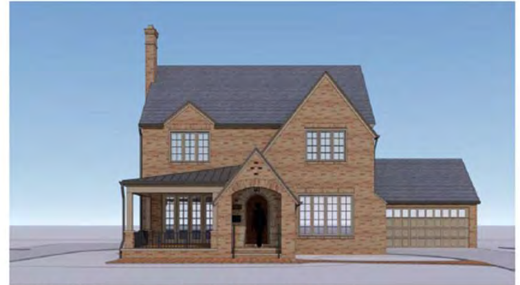
HIP ROOF - 1" Mini Batten, Standing Seam Metal Roof at 3:12, Color: Zinc Gray
