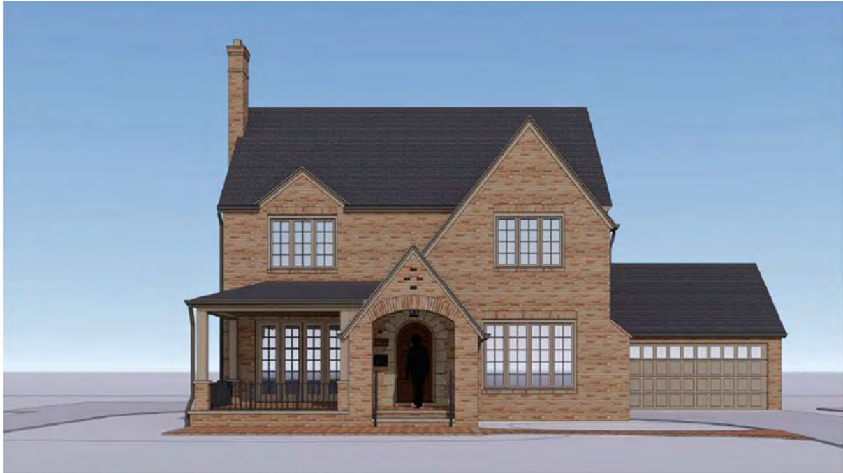
HIP ROOF - Asphalt Shingle, Certainteed Landmark, at 2:12, Color: Driftwood MAIN ROOF - Asphalt Shingle, Certainteed Grand Manor, Color: Stonegate Gray
