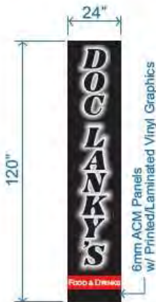
Double-Side Blade Sign (Existing Frame and External Illumination)
