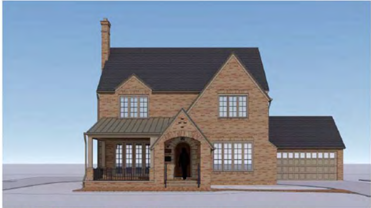
SHED ROOF - 1" Mini Batten, Standing Seam Metal Roof at 3:12, Color: Champagne Metallic
