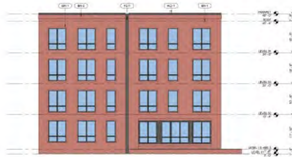
3 BUILDING SOUTH - WEST ELEVATION SCALE: 1/4" = 1'-0"
