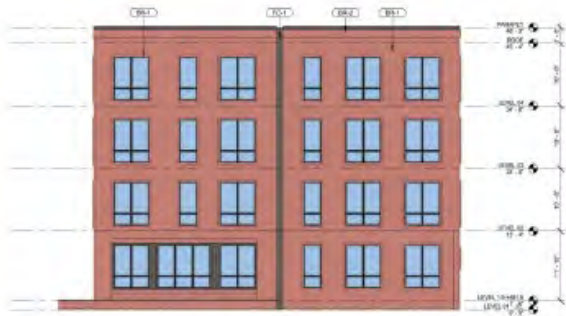
4 BUILDING SOUTH - EAST ELEVATION SCALE: 1/4" = 1'-0"
