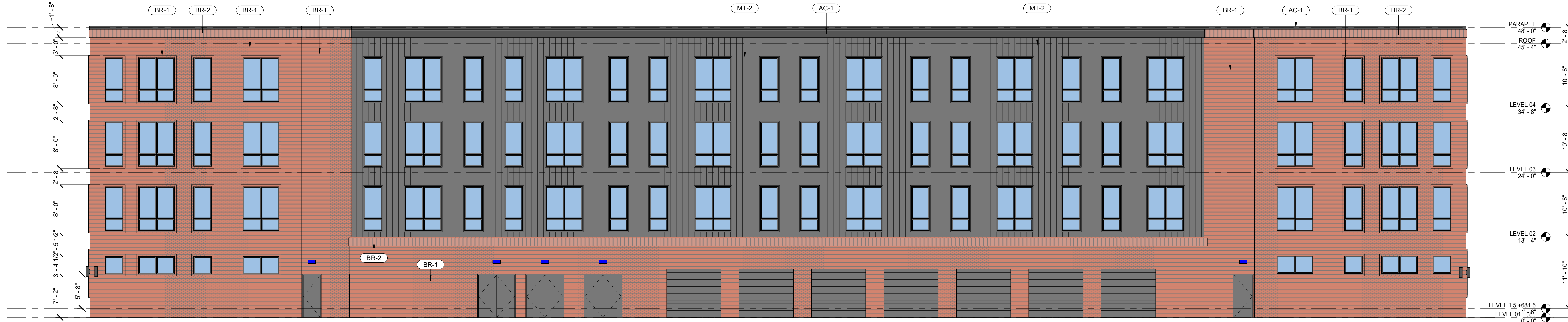
2 BUILDING SOUTH - SOUTH ELEVATION SCALE: 1/8" = 1'-0"
