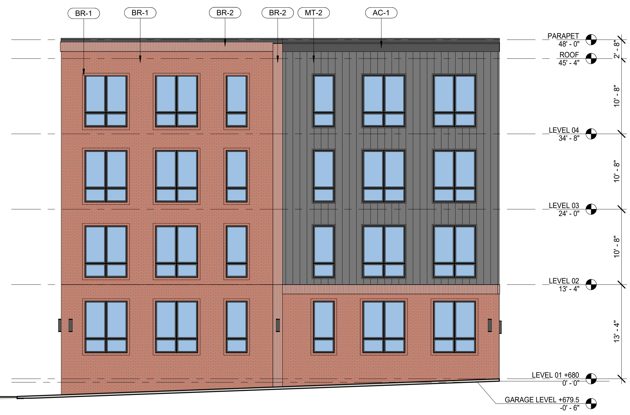
2 BUILDING NORTH - NORTH ELEVATION 2 SCALE: 1/8" = 1'-0"
