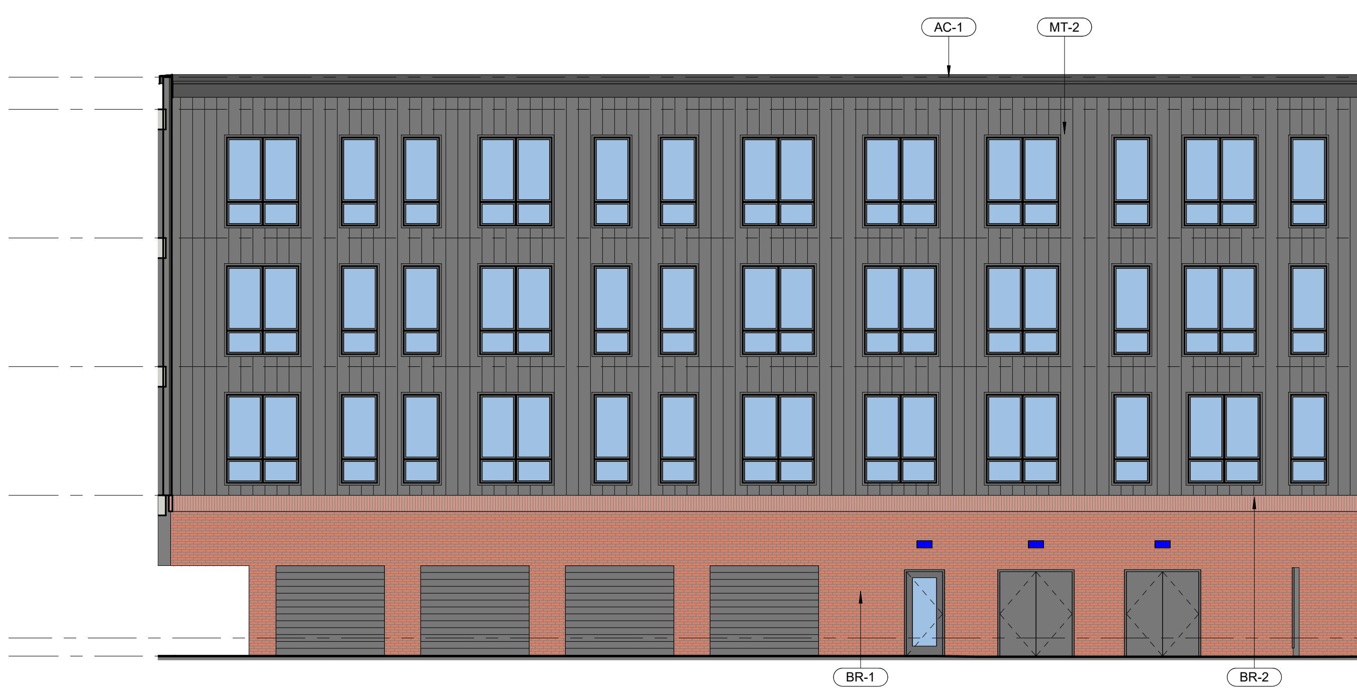
6 BUILDING NORTH - NORTH ELEVATION SCALE: 1/8" = 1'-0"
