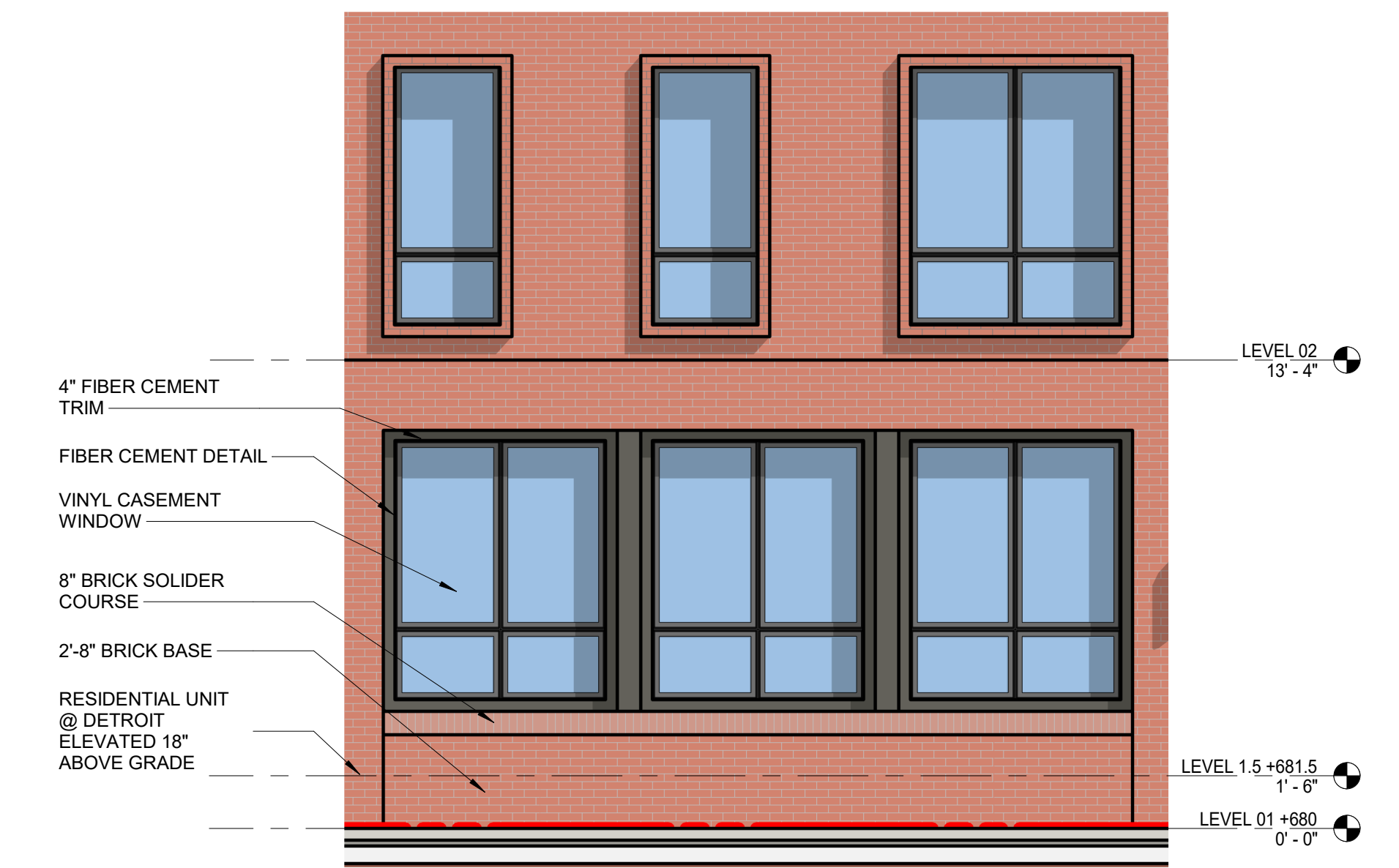
3 TYPICAL RESIDENTIAL WINDOW DESIGN - DETROIT AVE. SCALE: 1/4" = 1'-0"
