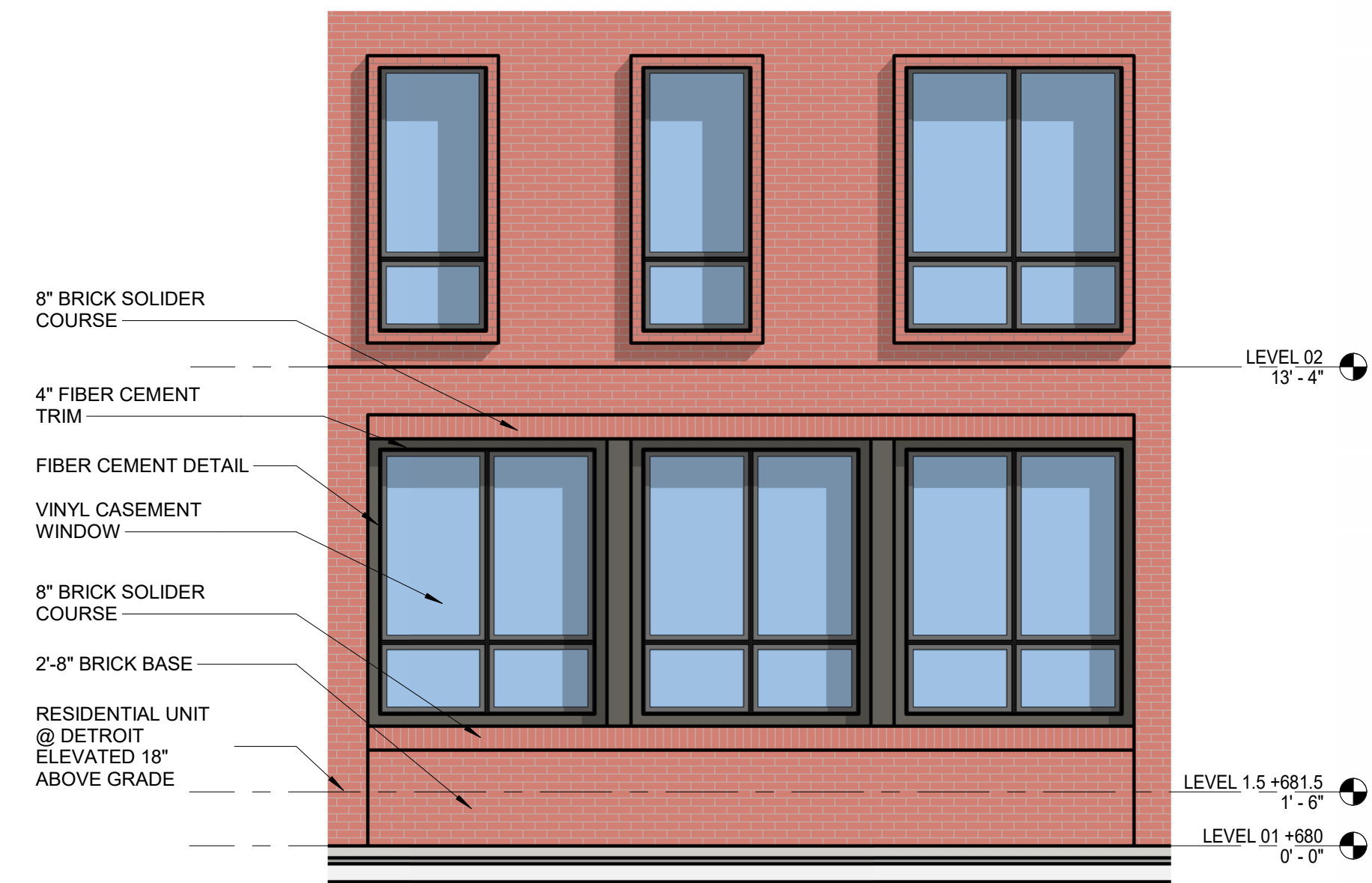
3 TYPICAL RESIDENTIAL WINDOW DESIGN - DETROIT AVE. SCALE: 1/4" = 1'-0"
