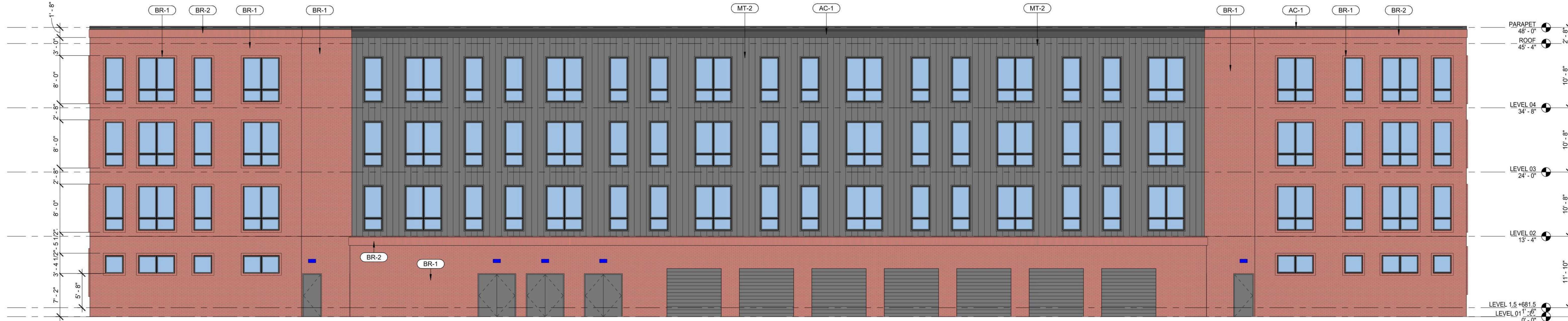
2 BUILDING SOUTH - SOUTH ELEVATION SCALE: 1/8" = 1'-0"
