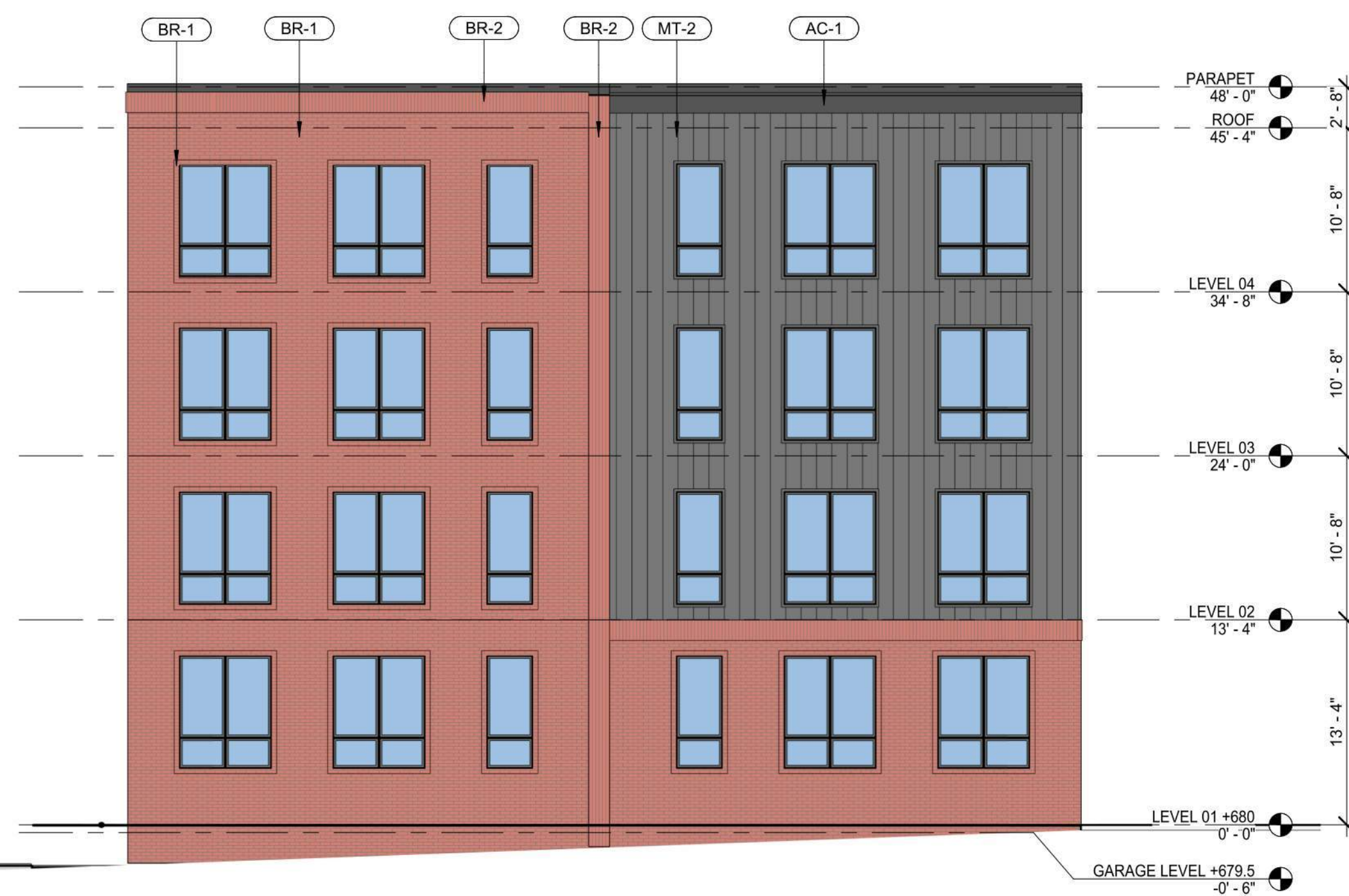
2 BUILDING NORTH - NORTH ELEVATION 2 SCALE: 1/8" = 1'-0"
