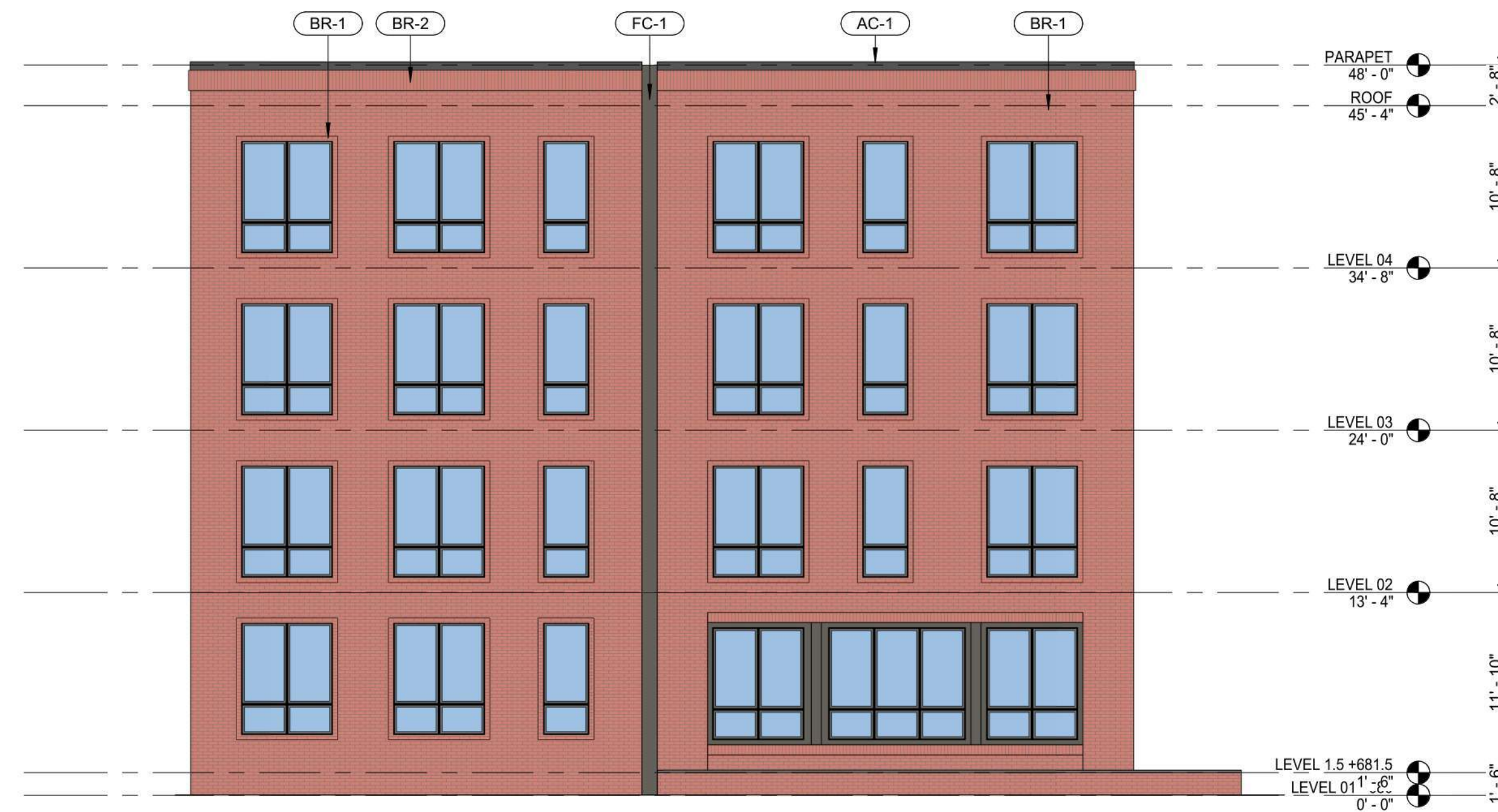
3 BUILDING SOUTH - WEST ELEVATION SCALE: 1/8" = 1'-0"
