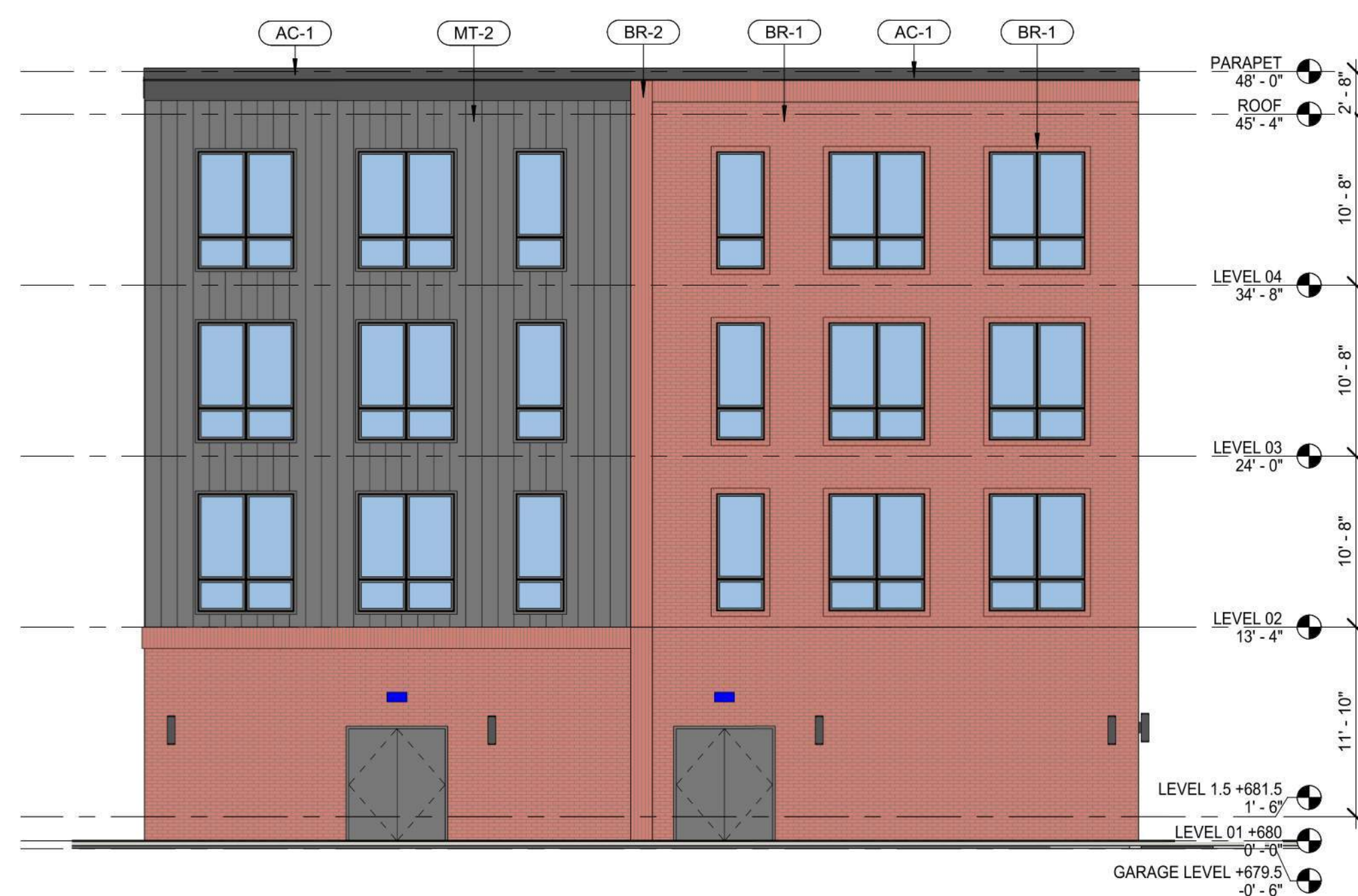
4 BUILDING NORTH - WEST ELEVATION 2 SCALE: 1/8" = 1'-0"
