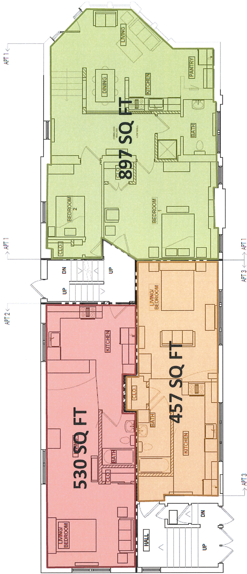
Proposed conversion of 1 st Fl. of Exist. Funeral Home into Three Residential Units
