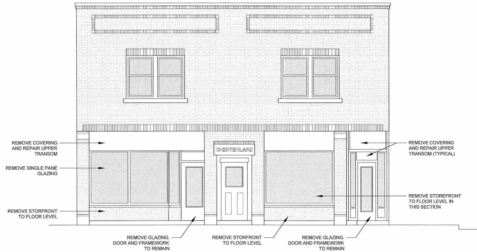
Existing Front Elevation
