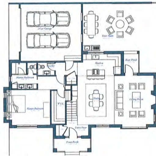
Unit A - Alt Scale: 1/8" = 1'-0" First Floor - 01 Room - 1,472 SqFt - 1,393 SQF - 1,471 SQF TOTAL - 01 Room - 1,472 SqFt - 1,393 SQF - 1,471 SQF Roomed Figure Footage - 1,393 SQF Garage Figure Footage - 80 SQF
