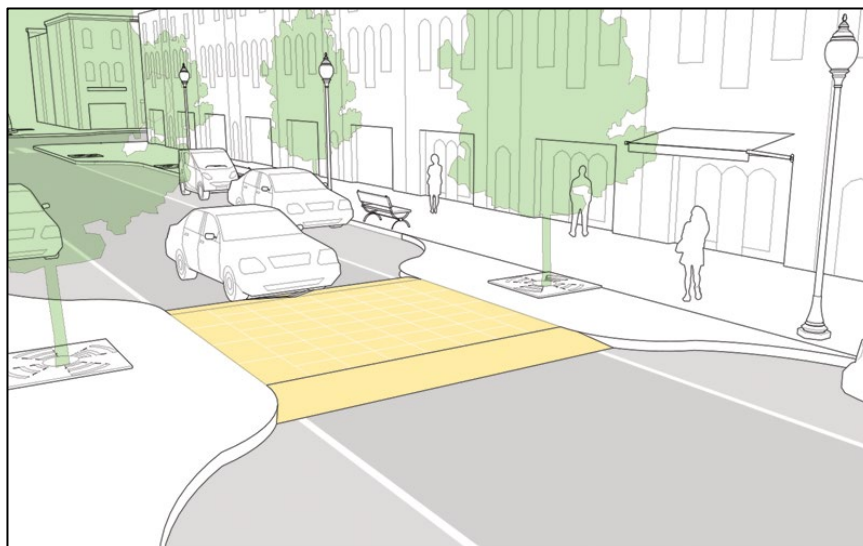
Figure A-8: Example Mid-Block Choker & Speed Table Combination (Source: NACTO Urban Street Guide)
