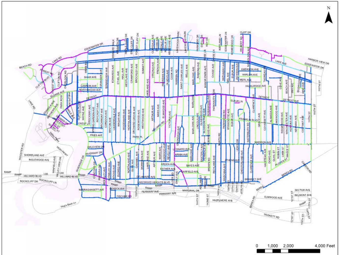
Figure 2-6. Water Main by Installation Year
