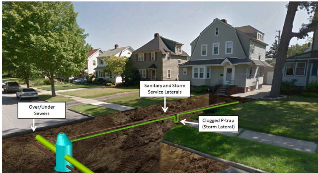
Figure 7-10: Existing Conditions in Over/ Under Sewer Areas
